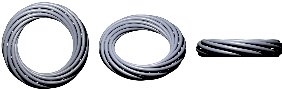
Figure 7: A nine-ring Villarceau coil
